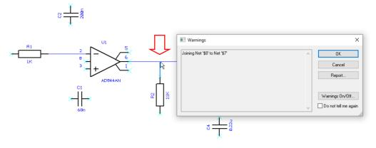
In the example above, this dialog warns you that the net \$8 is about to be connected to the existing \$7 and renamed. Yours may show slightly different net names. The \$ names are automatic net names created by the system and can be renamed at any time anyway.
