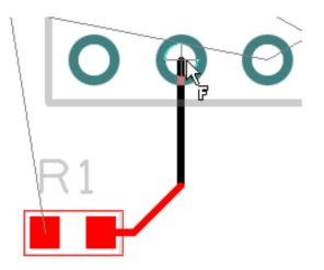
If you move the cursor over the target pad and hover, a modal cursor (a modified cursor showing the current mode of operation) will be shown. A single click when this is shown will finish the track
