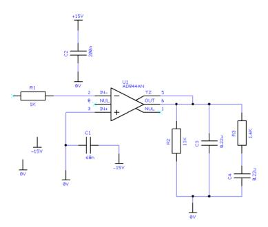
There is one more +15V Signal Reference symbol to add. If the symbol (or a component) exists in the design, you can simply copy it.
