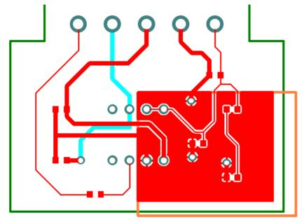
Now when you use **Pour Copper** from the context menu for the selected Template, the area will be flooded with copper that has thermal connections and isolation gaps on the OV nets.
