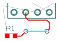
Pulsonix will insert a via at each end of the selected track segment and will swap the track to the Bottom layer (now drawn in blue).
