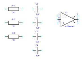
Before we make the connections we should change the **Component values** to be the ones required. This is easy to do because we've used 'generic' resistor and Capacitor components.
