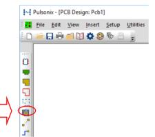
The shape may be created on the design. The Template may be drawn outside the board outline but Pulsonix will pour the copper using the Technology rules.
