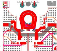
Irregular spiral shapes can be created using joining the two footprint pads. By the Pulsonix Embedded Component option defining the footprint as embedded, the Component can be mirrored in situ and all the inner layers will swap as required. Special DRC properties also allow the checking of correct internal connectivity made on the elements of these components.
