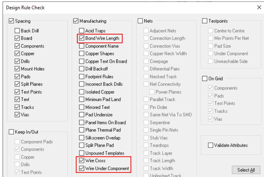
Minimum and maximum **Bond Wire Length** of the bond wires between bond pads and die pads. These rules are defined in the **Technology File** under the **Spacing Rules** tab
