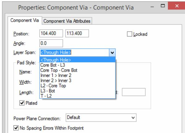
During creation, using the **Properties** for the via, these can be defined using the flag **No spacing check within footprint** set so that they can join two pads without any DRC errors when checked (for an embedded resistor via for example).
