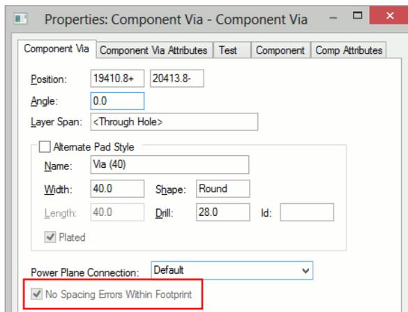
A Component Via is a fixed part of a footprint, but unlike a pad or mounting hole, it exists on a **layer span**, like a normal routing via. When defined, if this footprint is not marked as an Embedded Component, mirroring the component would not swap the inner electrical layers. By defining the footprint as an Embedded Component, you can mirror the component and all the inner layers will swap as expected.
