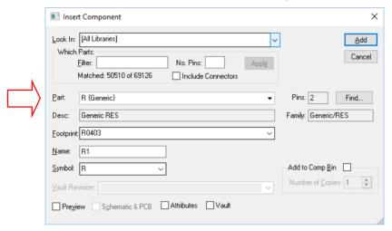
You will have a resistor selected with the first one to call named R1. By pressing the Preview check box, you can view it before it enters the design. Selecting the Schematic & PCB check box will enable both design previews of the Part chosen.
