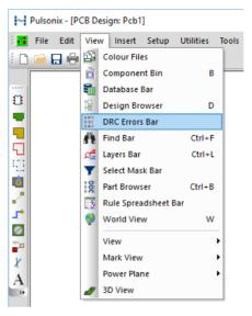
The **DRC Error Browser** is used to view all the design error makers as a sorted list. This list is displayed in an 'active' browser. Double-clicking in the list will select an error of which the error marker will be displayed in the design. The error marker will be brought into the centre of the display so it can be seen.
