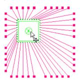
Once your bond pads have been correctly positioned, you can move the Die independently to reposition the die body, (a Die is considered to be a collection of Die pads within a component). To do this use the **Move Chip Body** option from the context menu of a selected component, this will move the 'chip' body without moving any of the Bond pads. Again, this option is only available as part of the Advanced Technology option.
