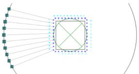
This option is used by selecting the Bond pads to place, then selecting the shape on which to place them around. The pads automatically snap to the shape but may need the placement grid to be corrected to fall exactly on the shape outline. You can use any shape but radial shapes provide the best results.
