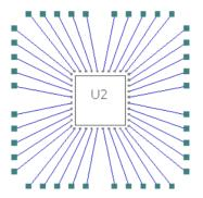
Once in the PCB design, and provided you have the **Advanced Technology** product option, the components act differently. Bond pads have the ability to move or 'float' independently of the Die pads or normal pads of the component (Die pads and normal pads are fixed within the footprint).
