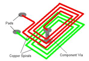
Planar Converters or Planar Transformers are possible using the Advanced Technology option.
