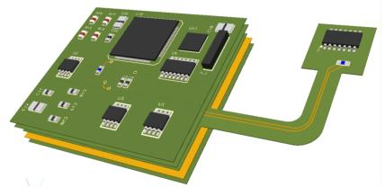
Both board outlines and board area cutouts can be assigned a layer span to support this.
