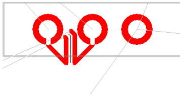
Without Keep correctly Paired checked. Tracks are allowed to be edited in illegally.
