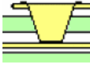
A Micro-via showing a tapered hole
