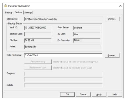
Restore existing – this will replace your current Vault contents with those contained in the backup. You do not have to have a Vault database prepared, one will be created from scratch as part of the Restore process, but you do need to have the Postgres database server installed and running. Use this option for normal restore of your existing working Vault.
