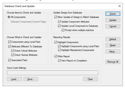
To start with, we will just see what the Check is going to report, so leave the Allow **Update of Design to Match Database** check box (in the top right corner of the dialog) unchecked, and check the all other options. Then select **Check**.
