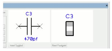
You can now either click Add then move the cursor into the design area and place your new component, or move the cursor over one of the preview boxes and 'pick and drag' the component into the design for placement.
