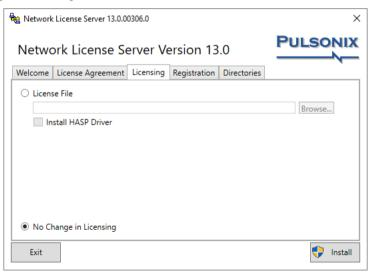
If you are using a USB key as your security device and this is a new installation, you may choose to **Install HASP Driver.** Setup will install the HASP driver for you. This is required in order for the USB key to operate. Do this before plugging in the USB key.
