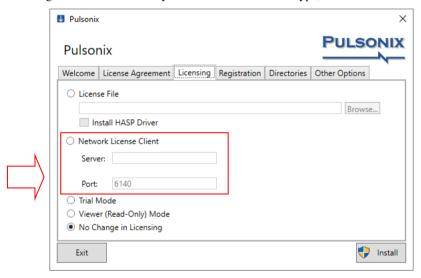
You are also requested for the **Server** name on which the License Server will run (or is already running). The License Server does not need to be running at the time, as the Setup program will not actually attempt to communicate with the server.
