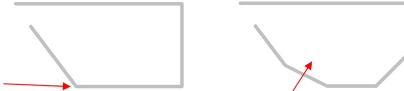
Leave it unchecked to only allow mitres between lines orthogonal and perpendicular to each other. This does not affect the Mitre Corner or Auto Mitre options.
