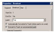
Note: These will get ripped out when using **Synchronise Design** if the switch in Design Settings (Allow PCB Only single pin nets) is not set on.
