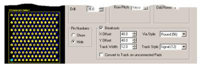
The X Offset and Y Offset allow you to create the direction of the breakout. The value entered in these boxes can be positive or negative numbers depending on the direction required. You can also specify the Track Width and Style required for the breakout as well as the Via Style if you wish to end on a via.
