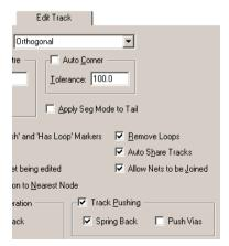
When **Spring Back** is enabled, pushed tracks will move back to their original position as the edited track is move away. **Spring Back** is recommended. It is also possible to push vias using the **Push Vias** option. This option will allow vias to be moved, you should be aware that moving a via may make it necessary to rework tracks on other layers.
