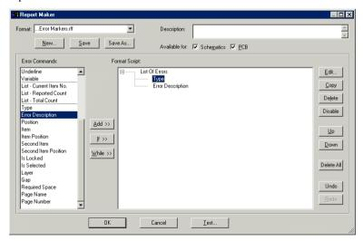
Various Commands exist for the error markers once the List Of Errors command has been used in the format script.
