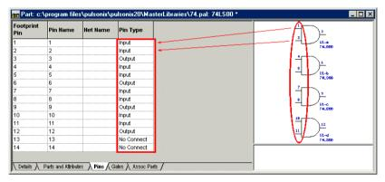
In the example above, after running the Match Pin Types option, the input pins and output pins have been allocated to their corresponding pin types.
