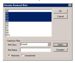
Once the Selection Filter criteria have been chosen (using the Net Class and/or Net Name choice), you click the Select button to make the selection in the top part of the window.
