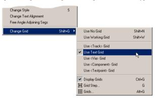
The current grid being used will be displayed on the status bar.
