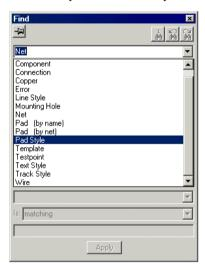
Items can be located by **Styles** for **Lines**, **Pads**, **Text** and **Tracks**. This is useful when trying to delete a style from the design to find what used it. Another use is to select all tracks for example that use a particular style, to change them all to a different style.
