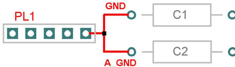
Even though the nets are physically joined at the star points, the nets remain separate and not merged. A special case for DRC is where the track segments attach to the star pad, and errors between these segments are not reported.
