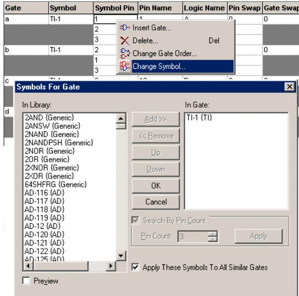
You can add additional gates to the list by using the **Add>>** button. The order in which these are listed will affect the order in which they appear in the Schematic design editor on the Insert Component dialog for example. The first one in the list will always be the one that is shown in these dialogs first.
