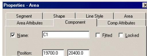
A **Fitted** check box has been added to the Component Properties page (and the Gate Component Properties page) this is only displayed if Variants are in use in the design and there is a 'Current' variant selected, (but not if Master Design is selected).
