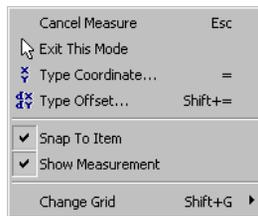
**Snap To Item** allows less accuracy on the picking of an item. This would be the normal mode of use. Leave it unchecked to restrict picking to positions in the design.
