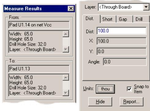
The dialog is shown split here for clarity. The top half displays dimensional information about the picked Items, or positions that the measurement was taken **From** and **To**. If there is more information that can be displayed, the vertical scroll bars are enabled to view all the data.
