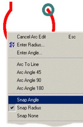
**Enter Angle** is used to type in an exact angle.
