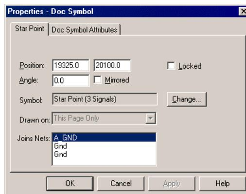
You can use the Properties dialog to **Change** the Doc Symbol and to display the net names (**Join Nets**) of nets connected to the star point.
