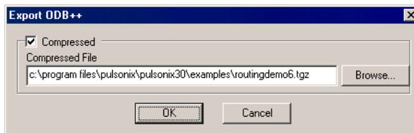
If Compressed is selected, it uses the TAR format and produces a single compressed file.
