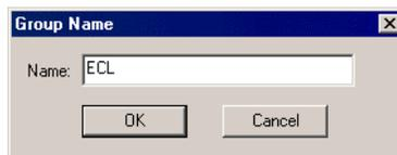
Groups can be named and the group and name passed through from Schematics to PCB designs. If the group is to be translated to PCB, it must be named. Named Groups can be managed using the **Technology** dialog and **Groups** tab.
