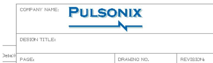
When used in the PCB design, the bitmap can be placed on any non-electrical layer. The layer change can be made using the **Change Layer** option. Design with Bitmaps inserted can only be plotted through the Windows output device they cannot be plotted to Gerber or ODB++.
