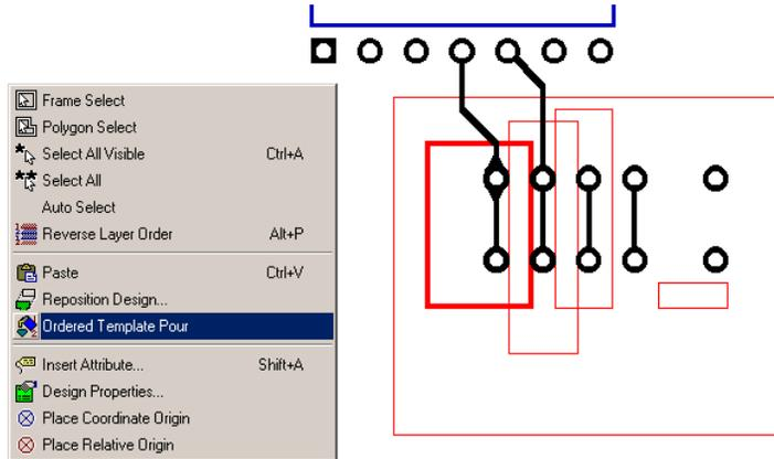
If no specific order is chosen, the templates will be poured in the order as added to the design. The order numbers are shown clearly for all templates in the design when this option is selected.
