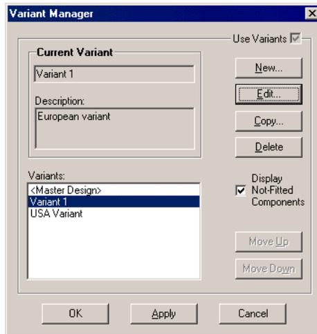
This allows variants to be enabled in the current design. Buttons for **New**, **Edit**, **Copy** and **Delete**, allow creation and manipulation of variants. The variant list order may be modified using the **Move Up** and **Move Down** buttons. Selecting from the list of variants will set the one selected as the **Current Variant** and is also displayed as a suffix, enclosed in brackets, to the design name shown in the design window title bar.
