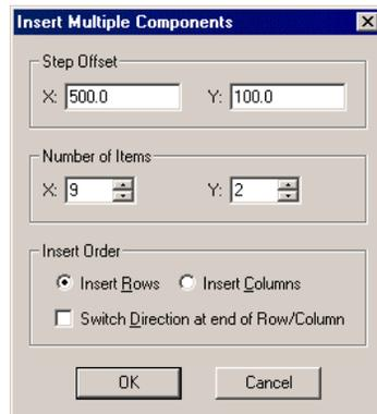
The **Step Offset** defines the distance each Component is offset from the previous one. There are separate values for X and Y and they may be negative to step in the reverse direction.
