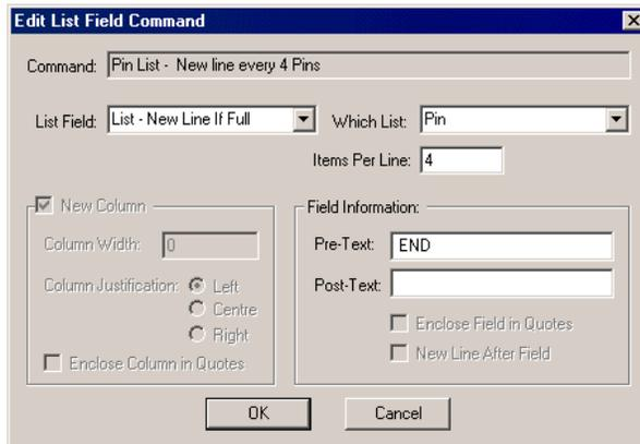
For some types of reports it is ideal to report the Component/Pin Numbers with up to 4 per line before starting a new line.
