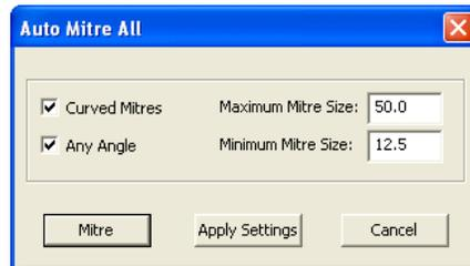
Use **Curved Mitres** to insert an arc instead of a line for the mitre.
