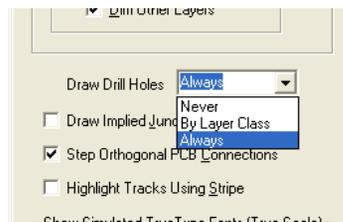
The **Draw Drill Holes** preference is only relevant to designs which can contain drill holes (e.g. PCB). It only affects drawing to the screen and not post processing. Redrawing speeds may be slightly enhanced by turning off drill holes (Never). The default is to draw drill holes when a displayed layer has a class with drill holes shown (By Layer Class). You can also choose to always draw drill holes when a pad is drawn (Always).
