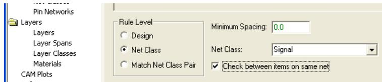
Only Tracks, Pads, Vias etc. are checked (copper is not checked). Tracks must connect directly to a pad (no corners inside the pad).
