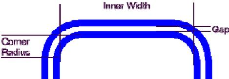
The spiral always begins at the inner right side and ends at the outer right side (but you can rotate or mirror it later).
