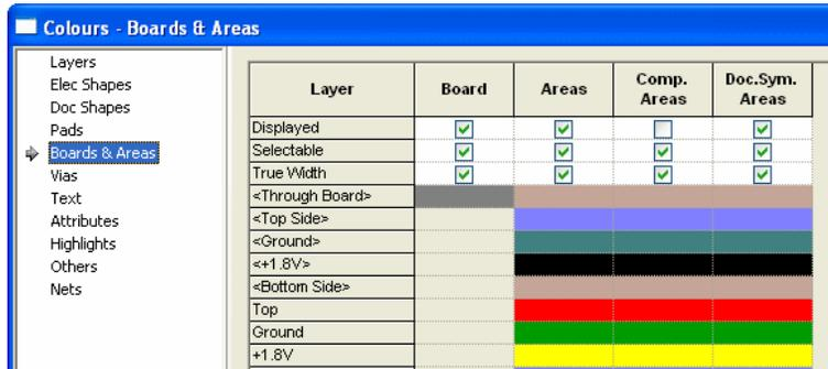
**Areas** has been moved from the **Elec Shapes** tab and **Board** has been moved from the **Others** tab. Both now appear on the new **Boards & Areas** tab that contains Layer Spans.
