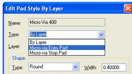
Normally, you would also do the same for the **Stop Pad** so the laser knows where to start and where to stop drilling, although this isn't mandatory for some processes. The Stop pad is displayed as a solid pad even though the default pad stack is defined with a drill hole, and the Entry pad is displayed with a drill hole shown (depending on Layer Class settings).
