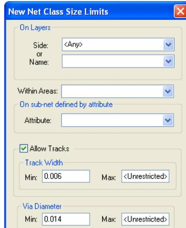
The **Net Class Size Limits** define restrictions on the widths of tracks and diameter of vias. They would normally be defined for critical nets in the Schematic then passed through to the PCB. This gives the Schematic engineer some control over how the net is routed. These rules are applied in terms of actual sizes, regardless of the Track and Pad Styles used.
