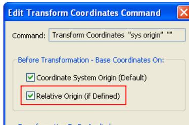
If **Relative Origin** is checked and the relative origin is placed in the design the coordinate will be output relative to it. Else, if the **Coordinate System Origin** box is checked and the system origin is defined it will be output relative to the system origin, otherwise it will be output using its exact value.
