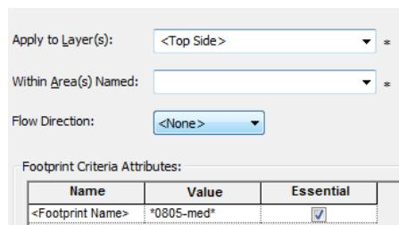
This scenario could also be used for swapping particular footprints in an **Area** by entering an Area name in the **Within Area(s) Named:** box.
