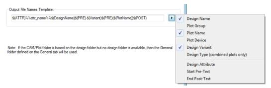
The **Design Attribute** keyword can be used to insert the value of design level attributes into the CAM/Plot and Report file names. This is available in the **Reports** dialog, **Cam/Plot Settings** dialog and the **Folders** dialog.
