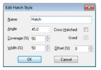
Using a Width: adjustment of 50%, the hatch line style is now 50% thinner than the template width.
