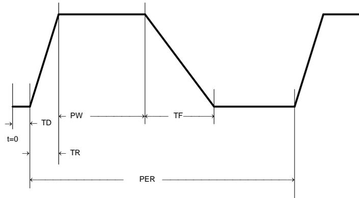
**Piece-Wise Linear Source****Schematic Entry**
