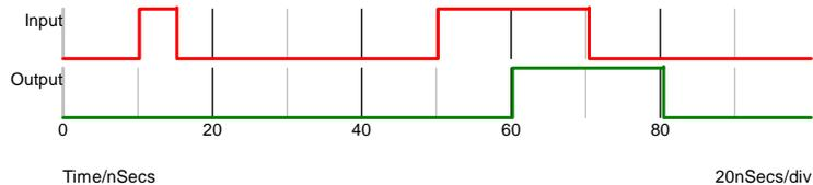
The Buffer device has an optional *stored delay* parameter that makes possible the specification of pure delays.
