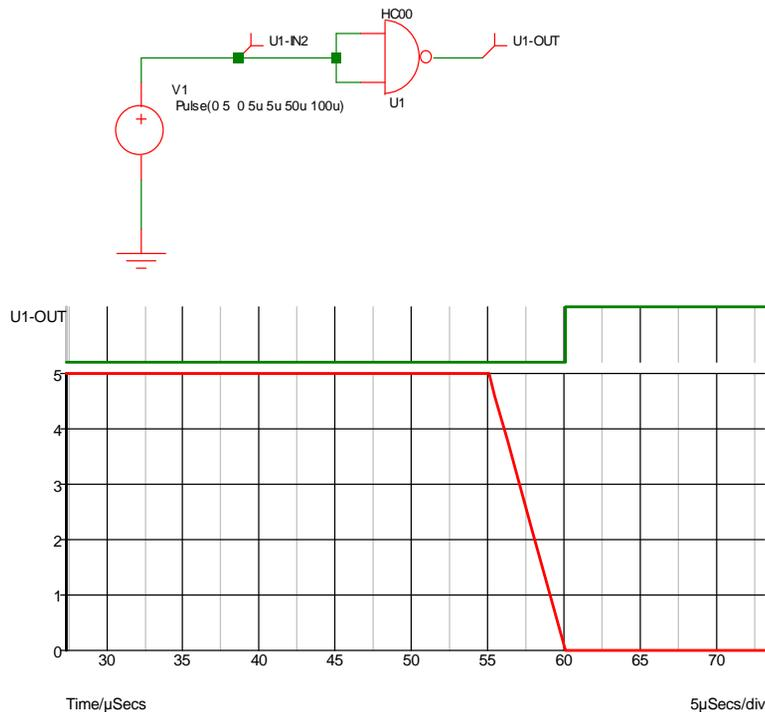
The graph shows the input and output of the NAND gate. Because the input is analog an implicit AD interface bridge will have been connected by the simulator. In the above example the parameters for this bridge have been set to:
