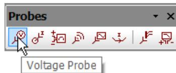
3. The voltage probe uses a single pin symbol, so you can release it on top of the connection required and it will automatically 'weld' itself to this net making itself fully connected.
