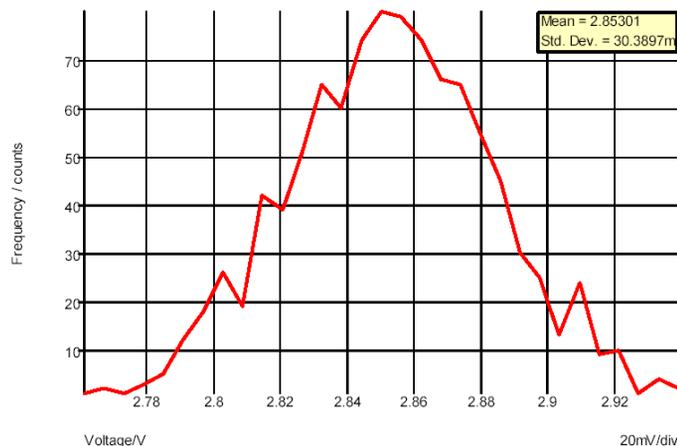
This is a histogram showing the distribution of the gain of the amplifier at 100kHz.
