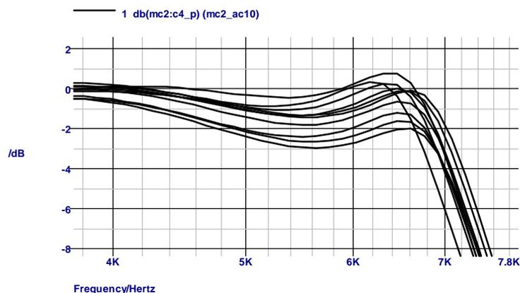
As can be seen, the specification is not met for some runs. Note that - as a rule of thumb - the spread for 10 runs will be about half of a realistic maximum spread ( $3\sigma$ ).
